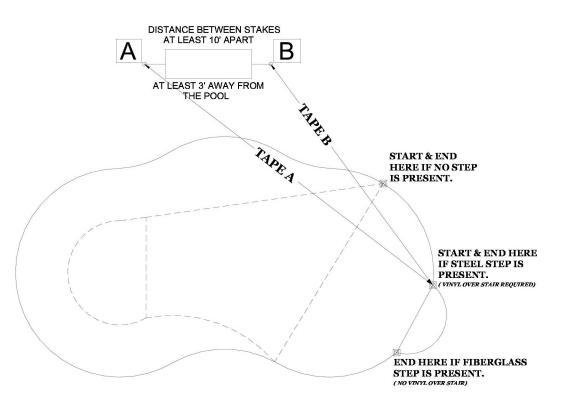
3. Attach a tape measure to each of the fixed stakes. Be sure to remember which stake is A and B (this is why two different color tape measures are suggested). Start from a definitive point on the pool such as the end of the step or the break-off. Pull both tape measures to the point at the same time. Record the measurement on the "A" tape in the A column on the measuring sheet and the "B" measurement in the B column. Ensure to record measurements to ¼ inch accuracy.
